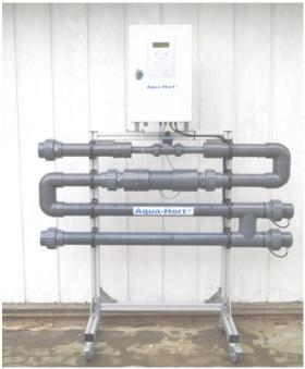
From below: two electrode pipes, then the electro magnet. The top pipe is the flow meter pipe. The control box is in front. Water in in the bottom pipe, and out of the top pipe.
