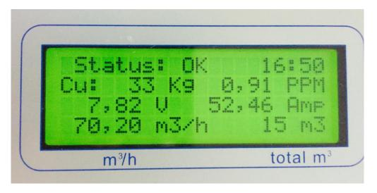
**The top line** of the display is showing to the left the Status of the system.
