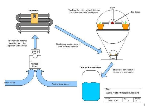
In cases where a placement after the fertilizer mixer is not possible, the Aqua-Hort is placed in the best suitable position, for example after a day tank with nutrition water, or in a inlet reservoir for the nursery. Nurseries with many fertilizer mixers might also be "forced" to choose this solution.
